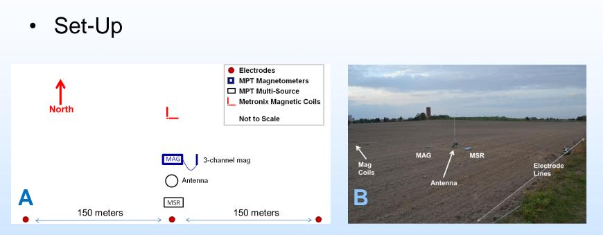
A) Map view sketch diagram of a typical field survey site and B)
